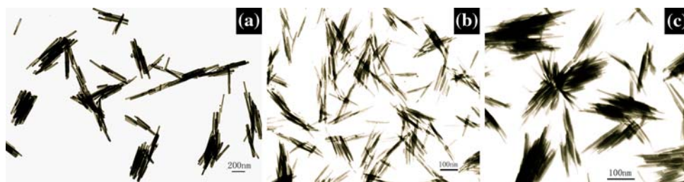
Fig. 6 TEM images of sample obtained at different concentration of the surfactant. (a) 10 CMC, (b) 100 CMC, and (c) 1000 CMC
